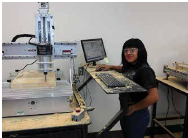
Michelle Carrillo, one of the high school students enticed to learn about manufacturing in the Cerritos College MTT program, monitors and waits for the CNC router to finish machining a guitar body. (PC with K2CNC software serves as the router's control.)
