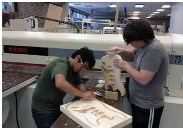
Alexis Estrada (left) sands the front side of his guitar body in preparation for set-up to machine the back, while Adam Mitchell, having machined both sides of his, smooths the step left by machining the second side.
