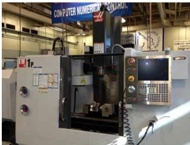
Nick Real, dean of technology at Cerritos, says this Haas 5-axis machining center, a recent addition to the metal shop, extends MTT instruction from virtual 5-axis programming and simulation to real 5-axis machining.
