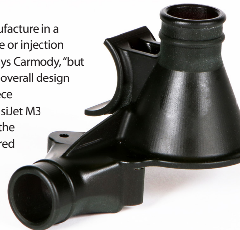
A single-piece housing for an air pump that integrates in and out flow points together with a mounting flange. The part was 3D printed in-house by evok3d on its 3D Systems ProJet 3500 HDMax printer using VisiJet M3 Black material.
