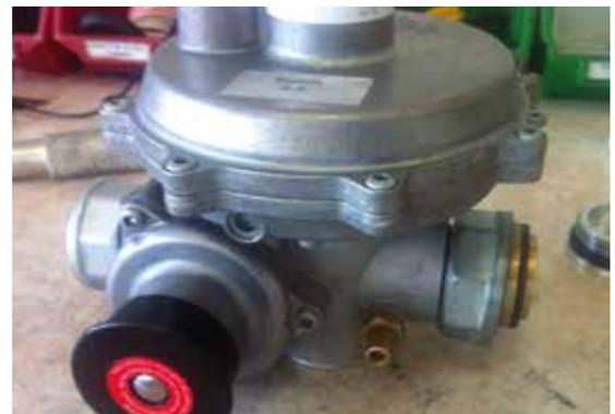
*Image above: Finished test model attached to regulator assembly*
