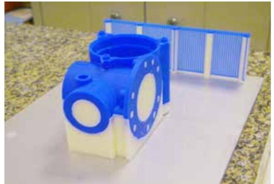
*Image above: One 3D printed wax part with white supports*
