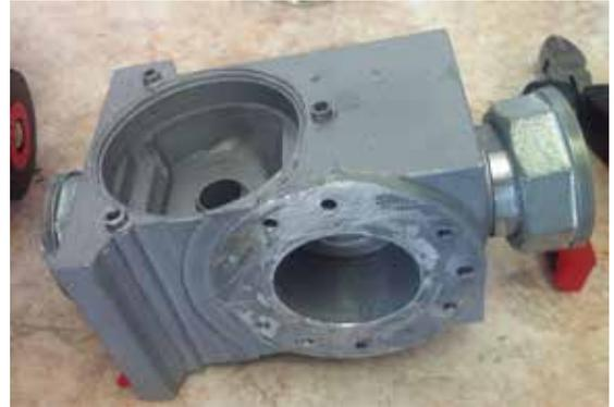
*Image above: CNC machined prototype didn't match Elster Aeroteh's requirements for testing*
