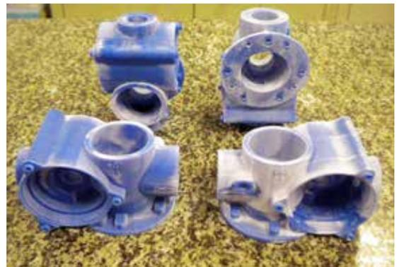
*Image above: Four wax models after cleaning and removing supports*
