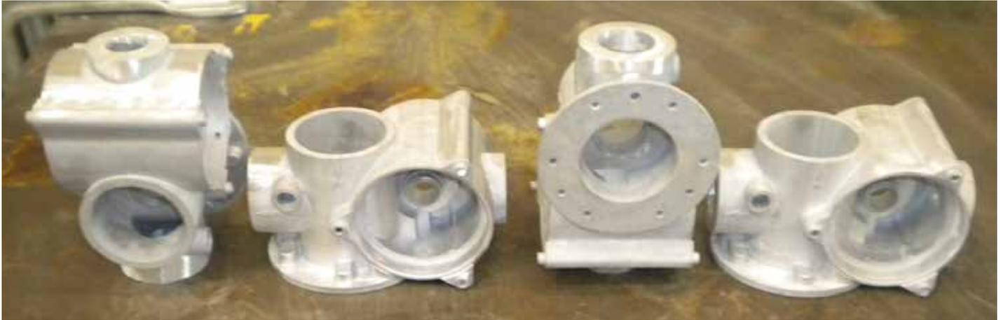
*Image above: Four final aluminum alloy pieces for testing*
