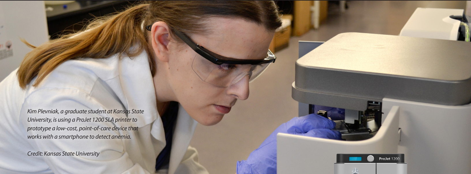
The ProJet 1200 provides a low-cost, high-speed alternative to prototyping a microfluidic point-of-care device.
