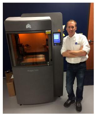
marker, to achieve a precision aesthetic shell, while the bulk of the part is filled-in with a much larger laser beam, which he likens to the wide end of the marker. This feature allows for a drastic reduction in build time as compared to previous-generation equipment that employs a single laser beam size. *(Left: Todd Resse with Realize Inc.'s ProJet 7000)*
