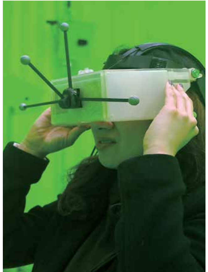
HEWDD-2 prototype 3D printed on the ProJet MJP 2500 Plus.
