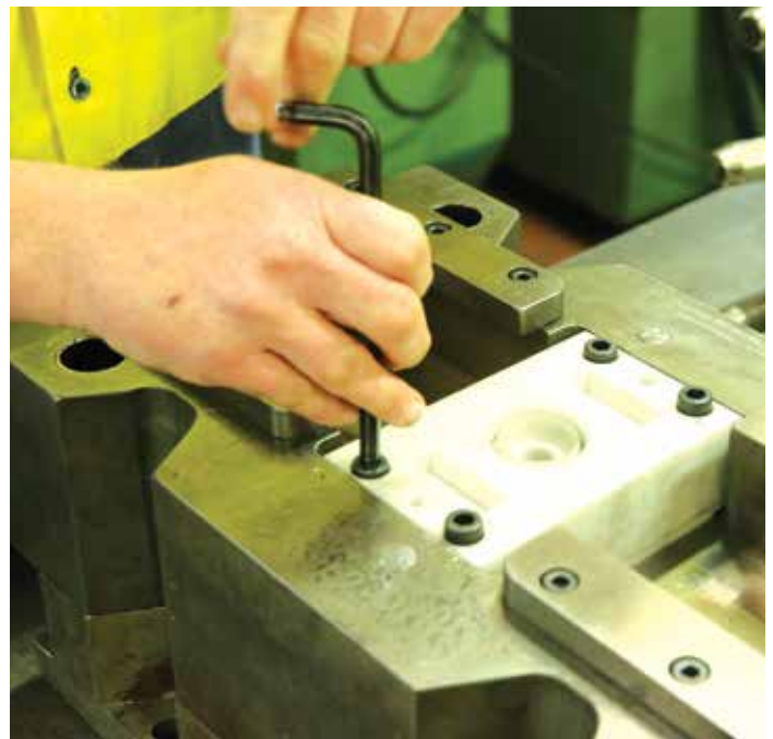
Time and cost considerations led Philmac to explore 3D printing for its production tooling prototype
