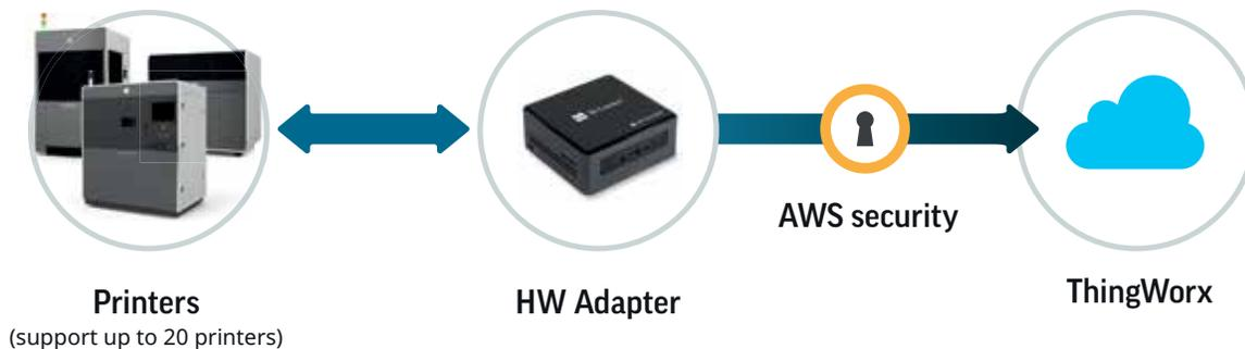
Data is collected from the printer(s) by the adapter, converted to an internal representation, and securely transmitted to an Amazon Web Services (AWS) hosted instance of the Thingworx platform (from PTC). 3D Systems controls and administers the Thingworx server. Only authorized 3D Systems employees have access to the AWS server.
