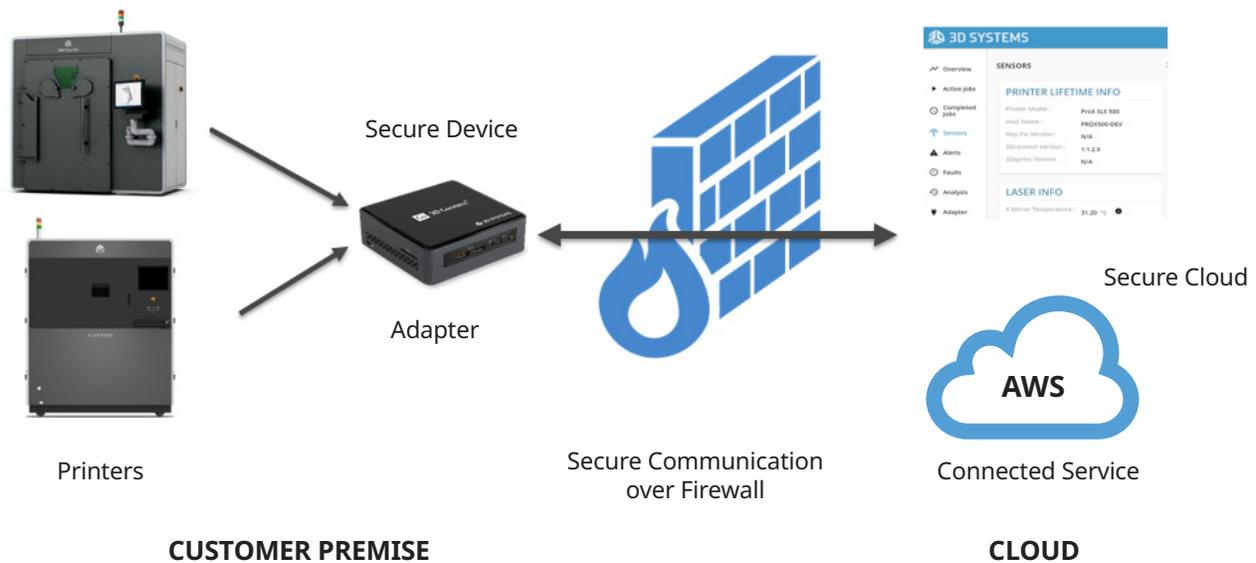
Printer data is collected by the adapter, converted to an internal representation, and securely transmitted to 3D Systems alert monitoring and data storage system hosted in Amazon Web Services (AWS). 3D Systems controls and administers the AWS services. Only authorized 3D Systems employees have access to the AWS server.
